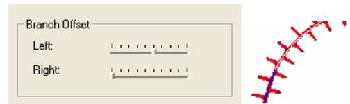
You can create joining stitch and stagger the stitching as well as control the stitch length and height.
